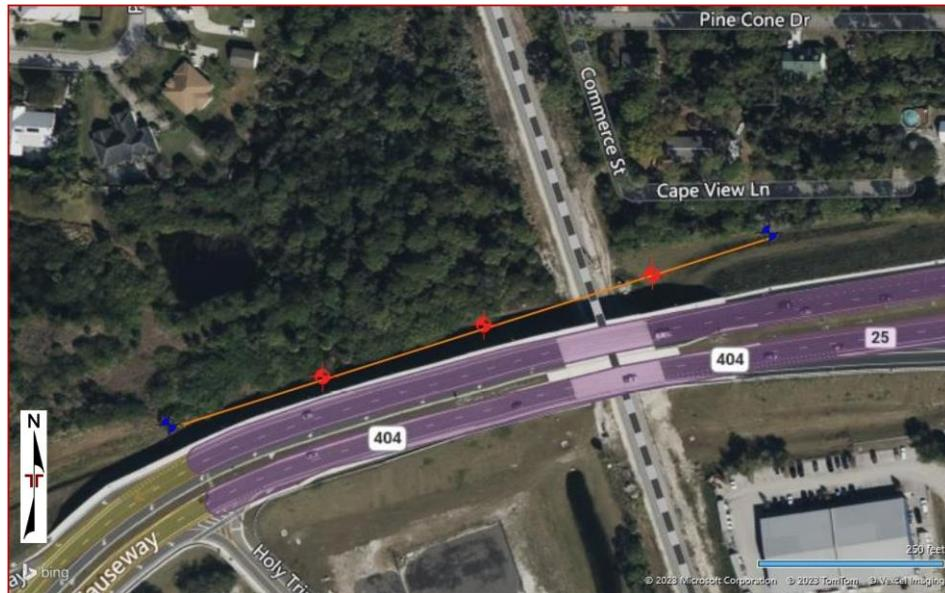
**Boring Layout:** Terracon will use handheld GPS equipment to locate borings with an estimated horizontal accuracy of +/-20 feet. Field measurements from existing site features may be utilized.
